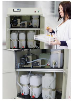
Application 3 Medical industry: automatic liquid mixing system, intelligent proportional mixing of different liquids, the system can intelligently detect the liquid level of the barrel. Through the analysis of the liquid state of each barrel, control the start and stop of the peristaltic pump, open and close OF solenoid valve, so as to realize the automation of the work flow.
