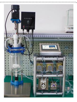
Application 4 Bio-pharmaceutical: Work with reactor or fermentation tank, the OCM system add different liquids with proportion and order into reactor. Together accomplish adding liquid, mixing, reaction, dispensing, waste discharge and washing function.
