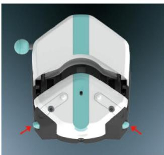
2. Turn the knob clockwise 180°, put the upper block back to original position, fasten the tube.
